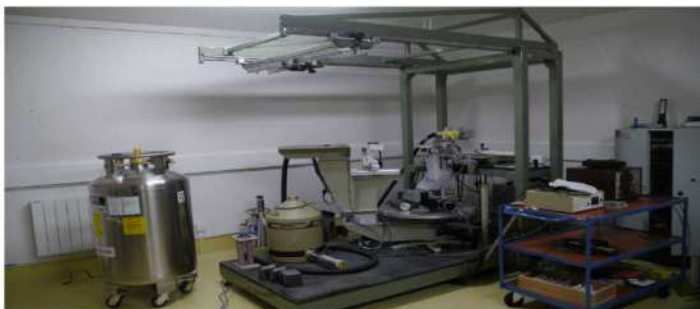
Multimodal Xrays bench (diffraction, scattering, fluorescence)
