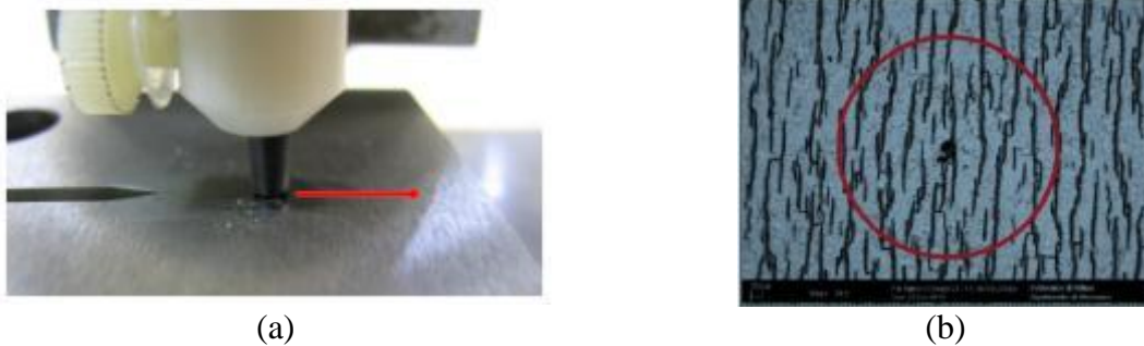
Figure 8: Inspection radius of the ET absolute probe: a) experimental determination by a cracked C(T) specimen; b) comparison of the inspection radius with the corrosion-fatigue damage pattern.
