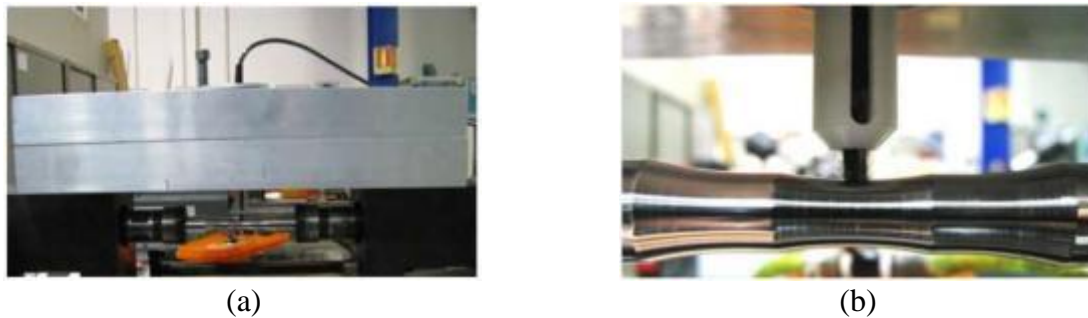
Figure 6: Application of the ET probes to small-scale specimens.
